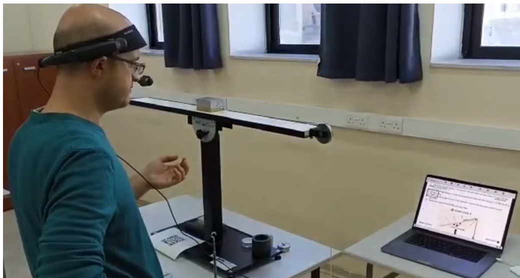
Figure 7: Voice Command to adjust the resolution: Zoom Level 3 and freeze window are two commands to zoom further into the document and lock the screen respectively.
